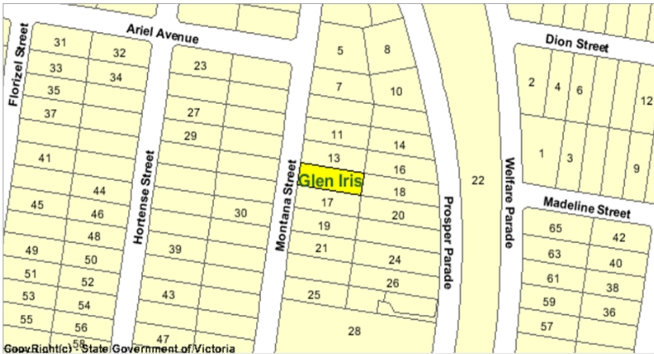
Figure 1 (above): Australian Capital Territory Digital Cadastral Database – survey accurate. Figure 2 (below): Victorian Digital Cadastral Mapbase (DCMB) – graphically accurate.
